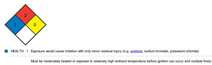
2 divided suspended solids that do not require heating before ignition can occur. Flash point between 37.8 and 93.3 °C (100
