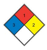
Short exposure could cause serious temporary or moderate residual injury (e.g. liquid hydrogen, sulfuric acid, calcium
