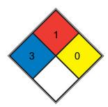
Short exposure could cause serious temporary or moderate residual injury (e.g. <u>liquid hydrogen, sulfuric acid</u>, <u>calcium</u>
