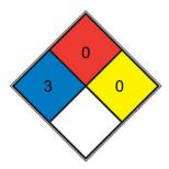
Short exposure could cause serious temporary or moderate residual injury (e.g. liquid hydrogen, sulfuric acid, calcium
