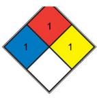
HEALTH 1 Exposure would cause irritation with only minor residual injury (e.g. acetone, sodium bromate, potassium chloride)
