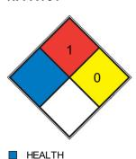
Materials that require considerable preheating, under all ambient temperature conditions, before ignition and combustion
