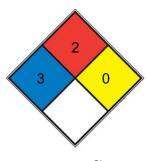
Short exposure could cause serious temporary or moderate residual injury (e.g. <u>liquid hydrogen, sulfuric acid, calcium hypochlorite</u>, hexafluorosilicic acid)
